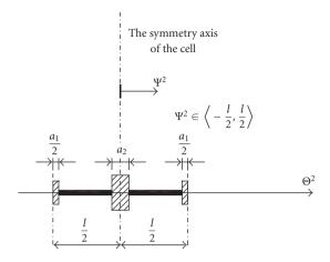
Figure 6.3. A periodicity cell along the  $O\Theta^2$ -axis direction on  $O\Theta^1\Theta^2$ -plane,  $a_1, a_2 \ll l$ .
