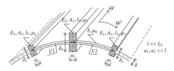
Figure 6.2. A fragment of the stiffened shell cross-section.
