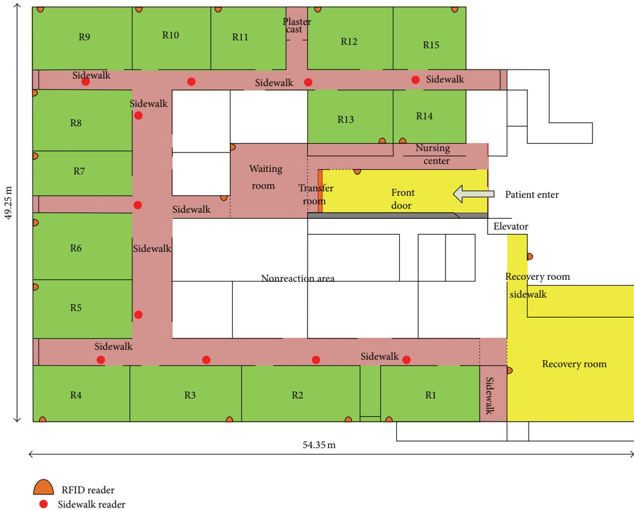
FIGURE 8: A simulated installation of RFID readers with 6-meters distance between two readers in the surgery room.
