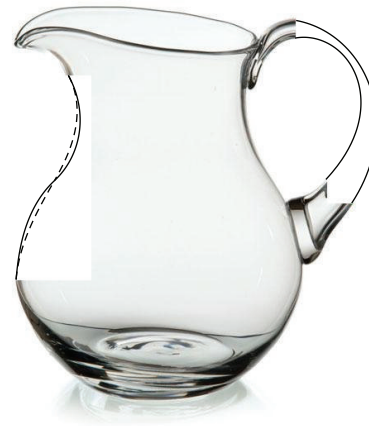
(b) LAC algorithm with two tangents setting for s-shaped curve and \alpha = -1
