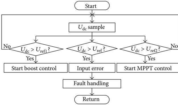
FIGURE 2: The DC/DC control flow chart.
