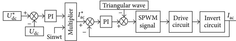
FIGURE 3: Double closed loop control block.
