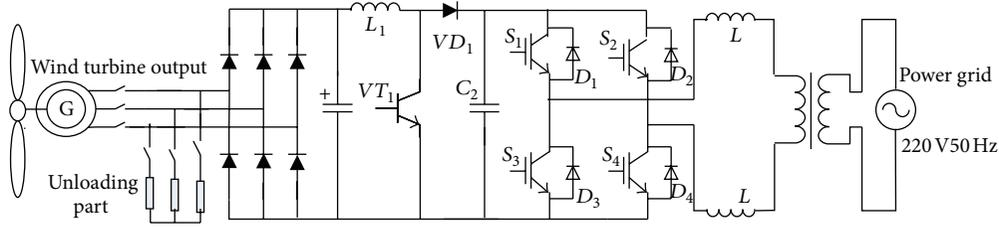
FIGURE 1: The topology structure of the small wind power generation system.
