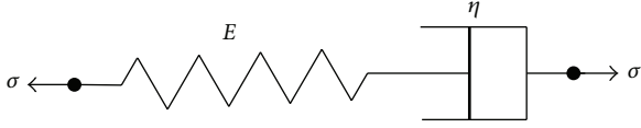
FIGURE 1: Maxwell model is made of springs ( E ) and dashpots ( \eta ) in series, and the forces acting on two parts are equal.
