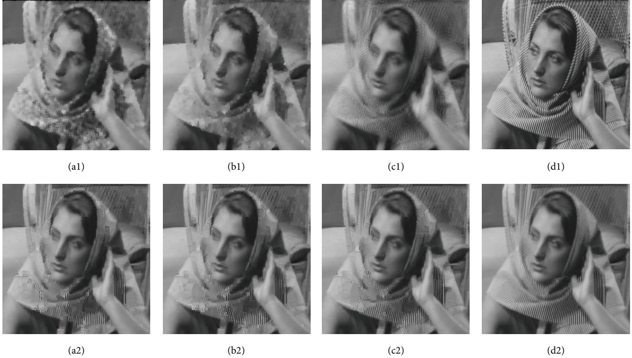
FIGURE 7: Denoised Barbara images with 50% salt-and-pepper noise. (a1), (b1), and (c1) are initial guide image using median filtering, total variation, and wavelet, respectively; (d1) original image; (a2), (b2), (c2), and (d2) are denoising results of the proposed method using (a1), (b1), (c1), and (d1) as the initial guide image, respectively.
