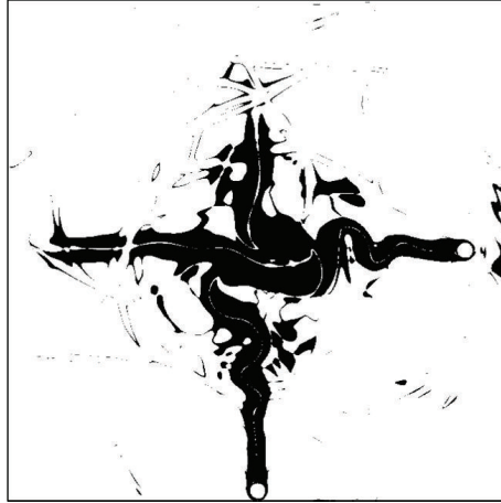
FIGURE 24: Visualization of switching parameter \beta at t = 23.2 with dx = 0.025D (white: \beta = 1 , black: \beta = 0 ).
