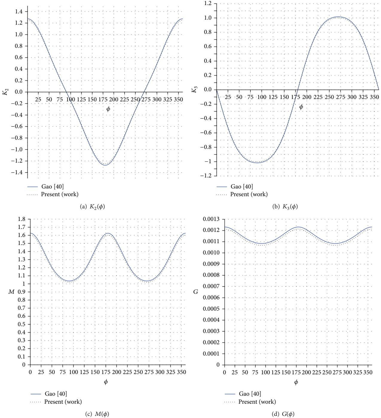
FIGURE 7: The  $K_2(\phi)$ ,  $K_3(\phi)$ ,  $M(\phi)$ , and  $G(\phi)$  for  $f(\zeta) = \zeta + c\zeta^3$  at  $c = 0.1$ .
