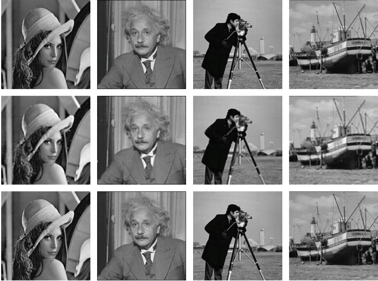
FIGURE 3: Images blurred with out-of-focus kernel of radius 3 and then corrupted by random-valued noise with noise level r = 55\% . Top: the restored images by MNID-ADMM and the parameters we used are [\alpha_1 = 0.002, \alpha_2 = 0.005, \beta_1 = \beta_2 = 0.02, \beta_3 = 5e - 6] . Middle: the restored images by Cai-TP. Bottom: the restored images by HADMM.
