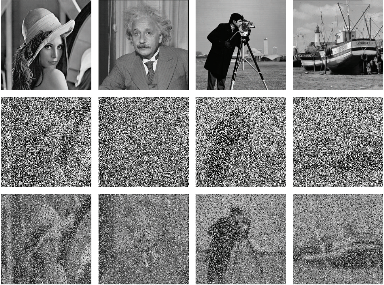
FIGURE 1: Top: the original images. Middle: Blurred and noisy images by using an out-of-focus kernel with radius 3 and corrupted by salt-and-pepper noise with noise level s = 70\% . Bottom: blurred and noisy images by using an out-of-focus kernel with radius 3 and corrupted by random-valued noise with noise level r = 55\% .
