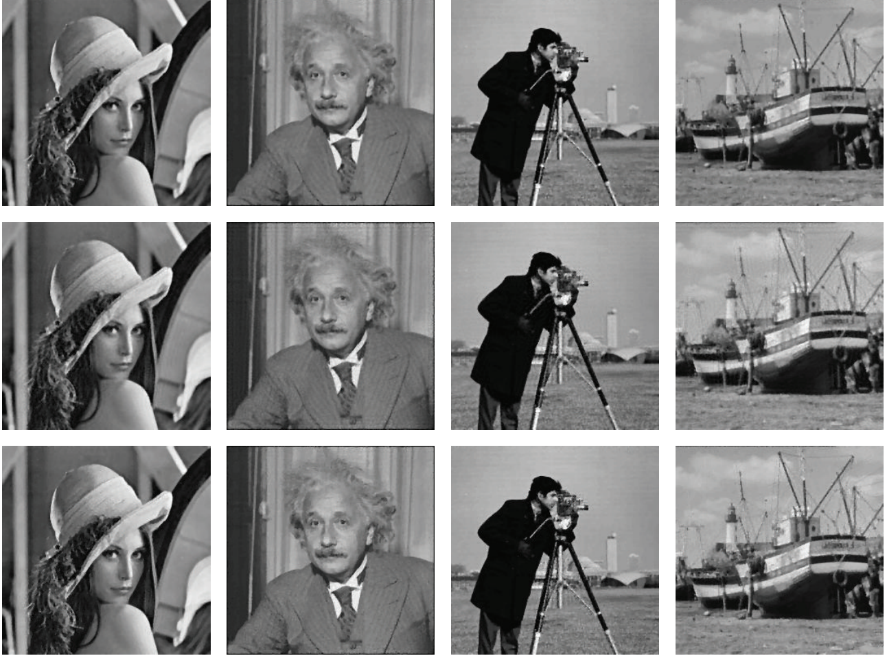
FIGURE 2: Images blurred with out-of-focus kernel of radius 3 and then corrupted by salt-and-pepper noise with noise level s = 70\% . Top: the restored images by MNID-ADMM and the parameters we used are [\alpha_1 = 0.01, \alpha_2 = 0.005, \beta_1 = \beta_2 = 0.01, \beta_3 = 5e - 6] . Middle: the restored images by Cai-TP. Bottom: the restored images by HADMM.
