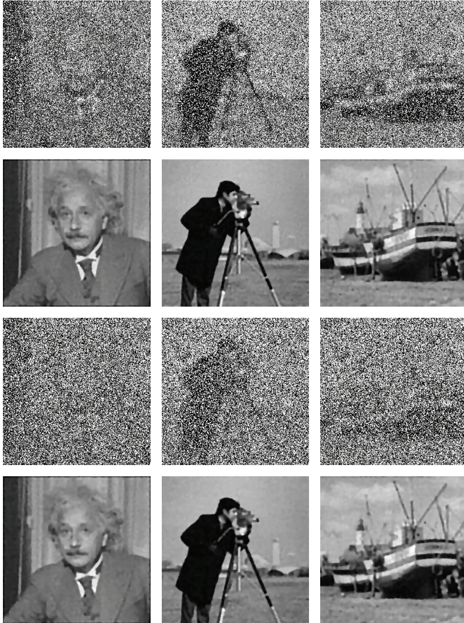
FIGURE 5: Top: images blurred with out-of-focus kernel of radius 3 and then corrupted by Gaussian noise with \sigma = 5 and salt-and-pepper noise with s = 50\% . The second line: results restored by MNID-ADMM ( \alpha_1 = 0.9 , \beta_1 = \beta_2 = \beta_3 = 0.05 ). The third line: Images blurred with out-of-focus kernel of radius 3, and then corrupted by Gaussian noise with \sigma = 5 and salt-and-pepper noise with s = 70\% . Bottom: results restored by MNID-ADMM ( \alpha_1 = 0.9 , \beta_1 = \beta_2 = \beta_3 = 0.05 ).
