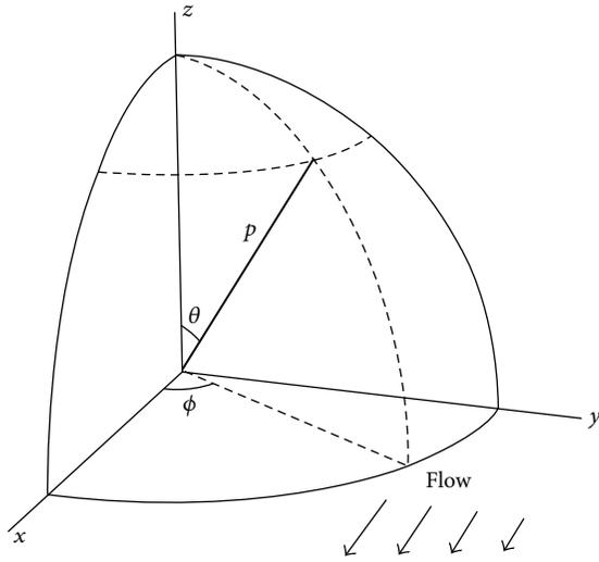
FIGURE 2: Schematics of fiber orientation. The bold line segment denotes the fiber orientation vector.
