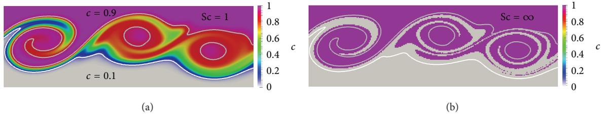
FIGURE 3: Comparison of instantaneous fiber concentration distributions (clipped). (a)  $Sc = 1$ , (b)  $Sc = \infty$ . Same isocontours of  $c = 0.9$  and  $c = 0.1$  for  $Sc = 1$  are also added in (b) for comparison purpose. The fiber concentration has a sharp front for  $Sc = \infty$ .
