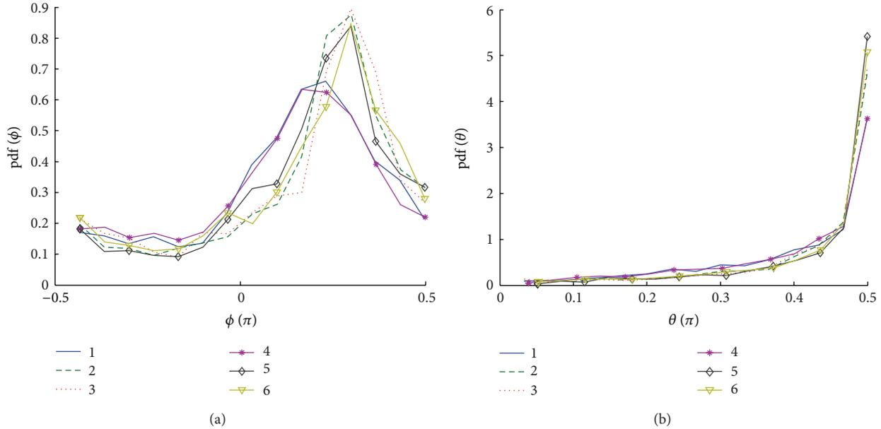
FIGURE 8: Orientation distribution at six positions: 1, 2, and 3 are at  $x^* = 228$  and correspond to  $\bar{c} = 0.3$ ,  $\bar{c} = 0.5$ , and  $\bar{c} = 0.7$ , respectively; 4, 5, and 6 are at  $x^* = 319$  and correspond to  $\bar{c} = 0.3$ ,  $\bar{c} = 0.5$ , and  $\bar{c} = 0.7$ , respectively. (a) Azimuthal angle  $\phi$ ; (b) polar angle  $\theta$ .
