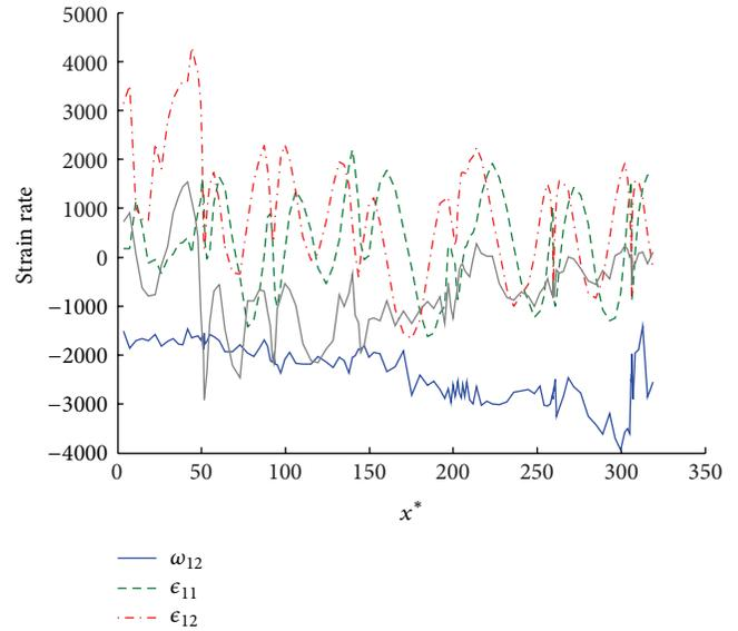
FIGURE 6: Profiles of the vorticity and deformation rate along a sample Lagrangian trajectory. The continuous gray is the corresponding determinant  $\Delta$  evaluated from (7).
