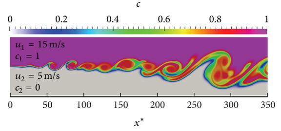
FIGURE 1: Schematic view of the mixing layer, with instantaneous fiber concentration  $c$  in the mixing layer for the case  $Sc = 1$ .
