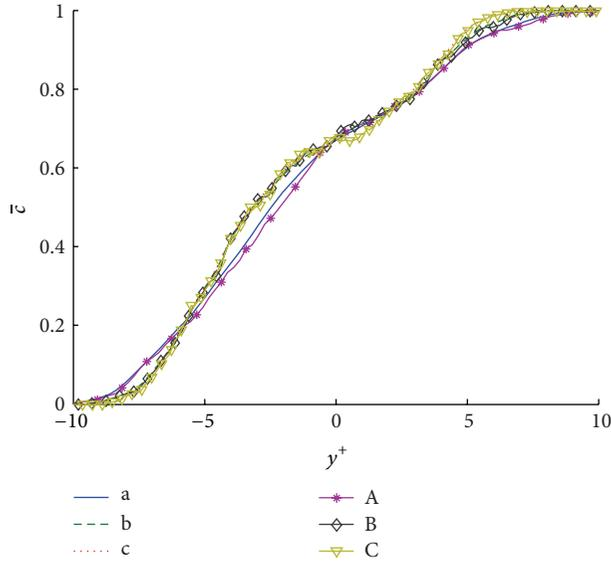
FIGURE 4: Mean concentration a cross profiles at various crosswise locations ( $x^* = 137$ ,  $x^* = 228$ , and  $x^* = 319$ ) for  $Sc = 1$  (a, b, and c) and  $Sc = \infty$  (A, B, and C).
