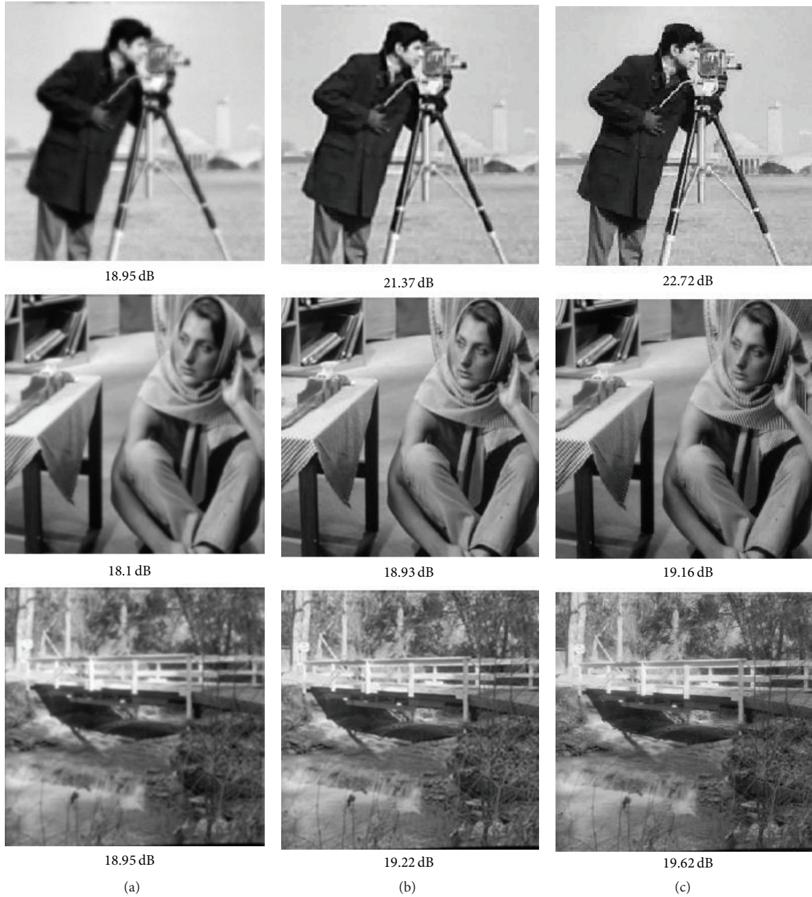
FIGURE 6: The blurred image (first column), the restored image by SGCS algorithm (second column), and HSG-V algorithm.
