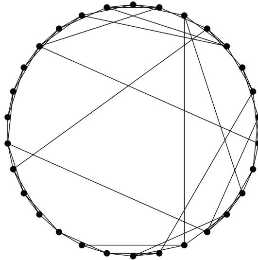
FIGURE 7: The structure of WS small-world network with  $N = 30$ ,  $K = 4$ , and  $p = 0.2$ .
