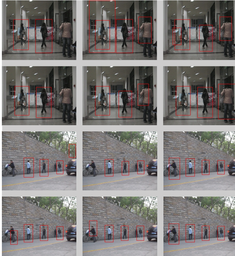
FIGURE 9: Detection results on XMU-VIS. From left to right and top to down, the classifiers are HOG_lin, LBP_lin, HOG.LBP_lin, HOG_HIK, LBP_HIK, and HOG.LBP_HIK.
