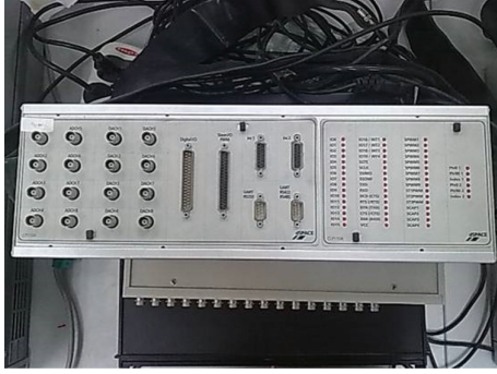
FIGURE 4: I/O interface board.
