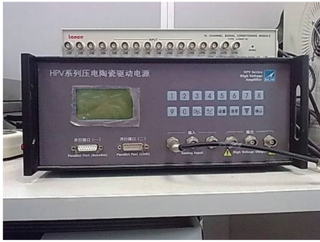
FIGURE 5: Piezoelectric driving power.
