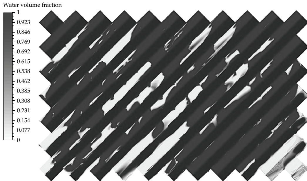
Figure 5: Typical liquid flow on surface of corrugation sheet.
