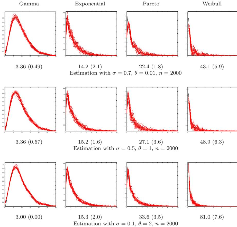
FIG 2. True density and 25 estimated curves. Estimation by deconvolution with sinc basis for different noise levels and different levels of the pile-up effect. Numbers below the figures indicate mean and standard deviation of the selected model  $\hat{m}$ .
