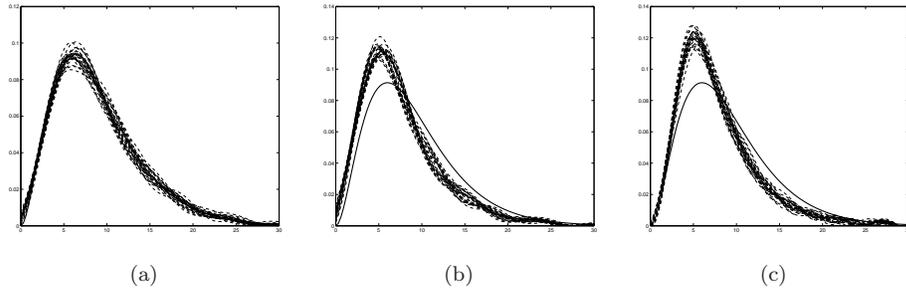
FIG 3. (a) Estimation with pile-up correction and deconvolution. (b) No pile-up correction. (c) No deconvolution.
