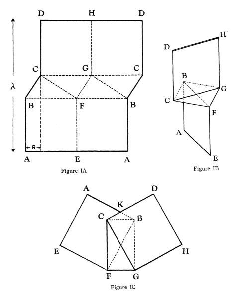
If  $\theta \neq 0$ , the point at the bottom of a generator must be identified with the point at the top of another generator, separated from the first by the angle  $\theta$ . The cylinder will be folded flat in such a way that at each end it is folded along two opposite generators, but the generators used at the top are displaced from those used at the bottom
