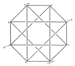
FIGURE 2. Top view of a realization of  $K_{4,4}$  in  $\mathbb{R}^3$  as a framework with two independent degrees of freedom. Vertices  $a_i$  are in the plane of the paper. Vertices  $b_j$  start out in a parallel plane above it, but do not remain coplanar as the mechanism flexes.
