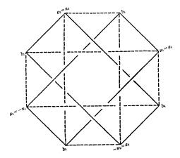
FIGURE 1. Top view of a realization of  $K_{4,4}$  in  $\mathbb{R}^3$  as a tensegrity mechanism. Vertices  $a_i$  are in the plane of the paper, vertices  $b_j$  in a parallel plane above it. Rods are solid, cables dashed.
