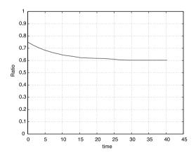
Fig. 3.3. Time variation of the ratio of the distance of the ball center to the cylinder axis and the radius of the cylinder.
