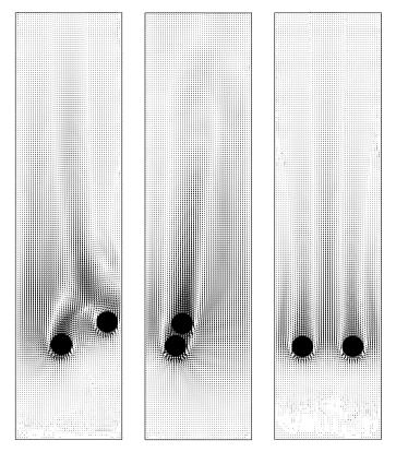
Fig. 3.5. Projection of the velocity field to the plane passing through the mass center of the left ball and parallel to the plane  $x_2 = 1/8$  at t = 1, 2 and 10 (from left to right).
