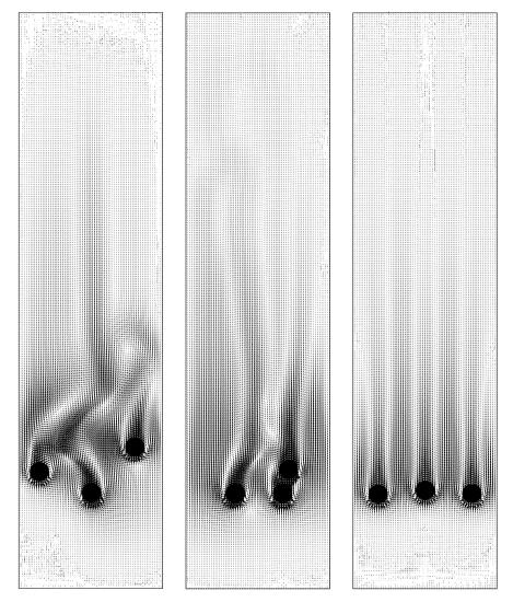
Fig. 3.8. Projection of the velocity field to a plane passing through the mass center of one of the three balls and parallel to the plane  $x_2 = 1/8$  at t = 1.1, 6.6 and 15 (from left to right).
