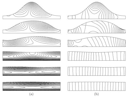
Fig. 4.6. Second test problem: the streamlines (left) and isobars (right) at times t = 0.05, 0.4, 0.75, 1.5, 2, and 2.5 (from top tp bottom).
