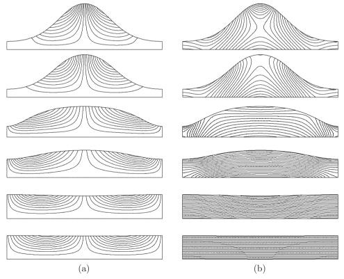
Fig. 4.4. First test problem: the streamlines (left) and isobars (right) at times t = 0.05, 0.15, 0.5, 0.75, 1.5, and 2.5 (from top tp bottom).
