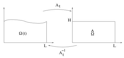
Fig. 4.2.  $A_t$  maps the current domain  $\Omega(t)$  onto the reference domain  $\hat{\Omega}$ .
