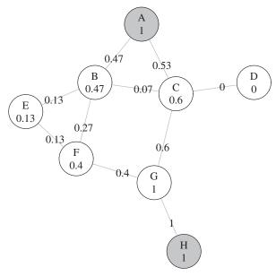
**Figure 2.** A resistor network with all resistances equal to unity (this is the same network of Figure 1). Each node is now labeled with the value of flow through it when a unit current is injected at node A and removed from node H. Each edge is labeled with the absolute current flowing on it.
