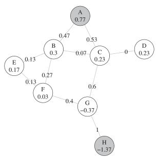
**Figure 1.** A resistor network with all resistances equal to unity. Each node is identified with a letter and is labeled with the value of its potential when a unit current is injected at node A and removed from node H. Each edge is labeled with the absolute current flowing on it.
