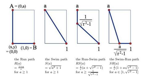
FIGURE 2. Possible optimal paths on the boundary of the domain and their time functions.
