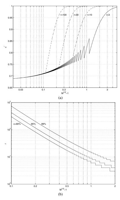
**Figure 1.** Behavior of optimum guaranteed confidence as a function of  $\sqrt{M} - 1$ : (a)  $c^*$  (dashed) and minimum  $c^*$  (solid); (b) minimum r that guarantees a confidence level.
