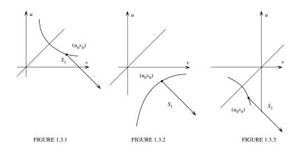
FIGURE 1.3. Shock waves emanating from  $(u_0, v_0), u_0 < v_0$ .
