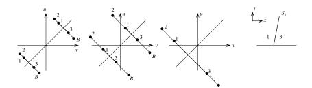
FIGURE 3.13. States' location and outgoing wave for  $R_2 + S_1$ .
