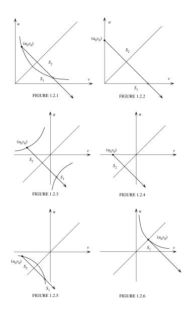
FIGURE 1.2. Shock waves emanating from  $(u_0, v_0), u_0 > v_0$ .
