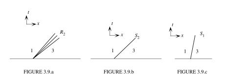
FIGURE 3.9. Outgoing waves for the  $R_2 + S_2$  interaction.
