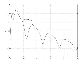
FIGURE 5. Graph of  $\|\Phi(t)\|_{\infty}$  for multi-mass vibration model with n = 5, resp. m = 10, plotted with  $\Delta t = 0.2$ .
