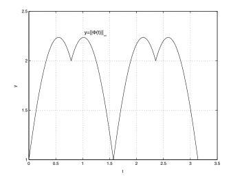
FIGURE 4. Graph of  $\|\Phi(t)\|_{\infty}$  for one-mass vibration model with  $\omega = 2$ , plotted with  $\Delta t = \pi/100$ .
