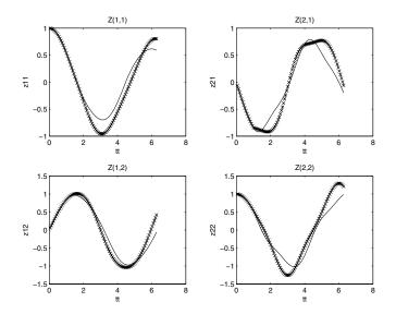
FIGURE 5. Four elements of the fundamental solution of the Van der Pol equation from 0 to  $2\pi.$
