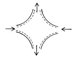
Figure 4. Sketch of boundaries of a rheometer. Arrows show flow direction of a viscous test fluid. A less viscous lubricant flows next to the walls.
