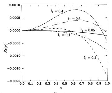
Figure 6. Growth rate versus  $\alpha$ .  $\Re$  for lower fluid =10, viscosity ratio  $\mu_1/\mu_2 = 0.01$ , density ratio  $\rho_1/\rho_2 = 0.95$ , surface tension coefficient  $/\mu_2 U^* = 0.1, U^* =$  dimensional plate speed.  $U^2/gl = 0.1, \ell$  dimensional plate separation.
