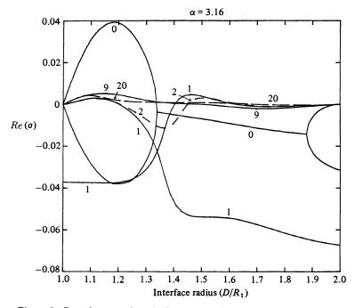
Figure 9. Growth rates when the less viscous fluid lies next to the outer cylinder.  $\mu_1/\mu_2 = 1.08$ ,  $\rho_1 = \rho_2$ , zero surface tension. Numbers next to graphs denote azimuthal mode numbers. The amount of the less viscous fluid decreases as  $D/R_1$  increases but various modes are unstable except when most of the gap is occupied by the more viscous fluid. At  $D/R_1 = 1$  mode 0 is at the first criticality and mode 1 is slightly below.
