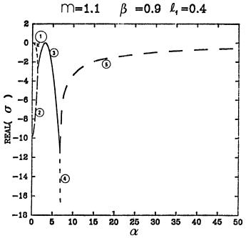
Figure 11. Growth rate versus wavenumber. Rayleigh number of fluid 1 is 1695.7, Prandtl number of fluid is 1;  $\mu_1/\mu_2 = 1.1$ ,  $\ell_1 = 0.4$ ,  $\hat{\alpha}_1 \Delta T = 0.001$ ,  $\Delta T =$  dimensional temperature difference between plate,  $\hat{\alpha}_1/\hat{\alpha}_2 = 0.9$ , surface tension = 0.
