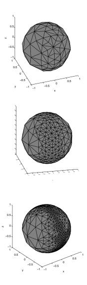
FIGURE 9. The first three adaptively generated meshes for  $V\dot{\varphi} = \dot{f}$  starting from an icosahedral triangulation with 80 nodes,  $\theta = 0.9$  [26].
