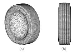
FIGURE 6. Discretization of car, respectively, truck, tires used for computations [16].
