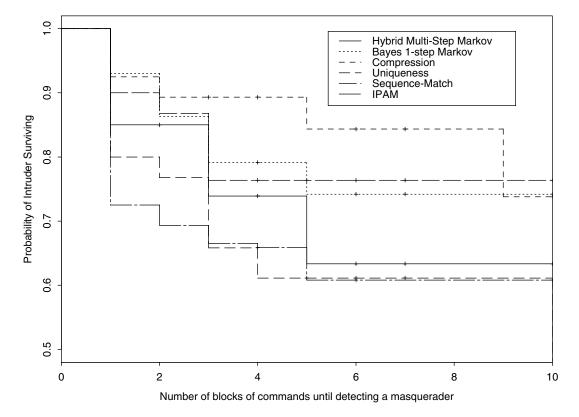
FIG. 5. Survival plot of intrusions for all methods given a fixed false alarm rate of 1%. Ideally there would be no detection delay, that is, instant "death" of the intrusion.
