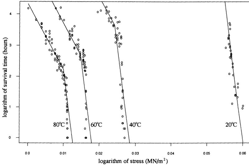
FIG. 3. *Data for plastic pipe.*
