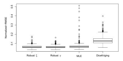
FIG. 5. Boxplots, for the four estimation methods, of the normalized RMSE for prediction of the Borehole function, based on n = 25 design points to build the emulator and averaging over N = 500 different designs generated from a Maximin LHD design. The average baseline MSE is 2079.36, using only the mean for prediction. The average MSE for the 4 methods (from the left to the right) are 9.07, 8,72, 14.77 and 41.29.
