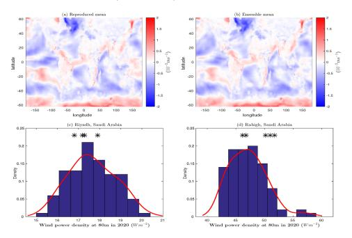
FIG. 7. Top: Global maps of (a) the mean from reproduced runs and (b) the ensemble mean of the near-future (2013–2046) annual near-surface wind speed trends. Bottom: Histogram of the distribution of the wind power density at 80 m in 2020 with nonparametric density in red for the one-hundred reproduced runs near (c) Riyadh and (d) Rabigh, Saudi Arabia (\* represents the original climate model runs).
