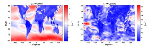
FIG. 1. The (a) ensemble mean  $\overline{\mathbf{W}}(2020) = \sum_{r=1}^{R} \mathbf{W}_{r}(2020)/R$  and (b) ensemble standard deviation  $\mathbf{W}_{sd}(2020) = \sqrt{\sum_{r=1}^{R} {\{\mathbf{W}_{r}(2020) - \overline{\mathbf{W}}(2020)\}^{2}/R}}$ , where R is the number of ensemble members, of the yearly near-surface wind speed (in  $ms^{-1}$ ) for R = 5.
