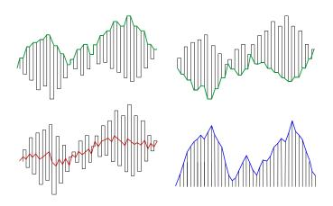
Figure 3: Example of the upper envelope (top-left picture), of the lower envelope (topright picture), of the middle line (bottom left picture) and of the profile (bottom right picture) of a given trajectory (in dashed line).
