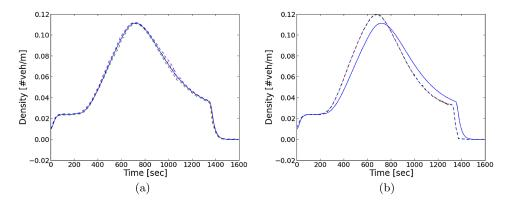
FIG. 12. Estimated density at cell 3. (a) With parameter learning. (b) Without parameter learning. The blue line on both plots is ground truth and the dotted line is the filtered value computed by the algorithm. The number of particles was chosen N = 1000.
