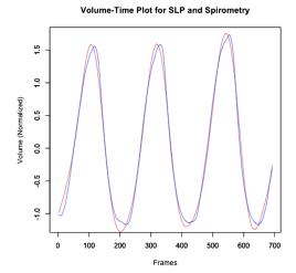
FIG. 2. Volume over time obtained using SLP and spirometry for an individual.
