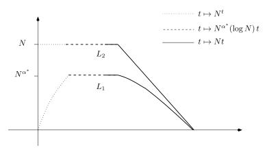
FIG. 1. A first-order picture of the network with  $\rho_1 + \rho_2 < 1$ ,  $\rho_1 < 1/2$  and  $(L_1(0), L_2(0)) = (0, N)$ . The first queue grows according to step (a), then the queue behaves as an OU process for a while according to step (b), then finally the system converges to zero according to step (c).
