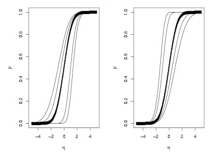
**Figure 2** *Response curves: Power Probit (left) for*  $\lambda = \{0.4, 0.6, 1, 4, 8\}$  *and Reciprocal Power Probit (right) for*  $\lambda = \{8, 4, 1, 0.6, 0.4\}$  *with different values of the linear predictor*  $\eta_i$  *and curves showed from left to right in both figures.*
