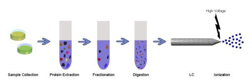
FIG. 2. Sample preparation. Complex biological samples are first processed to extract proteins. Proteins are typically fractionated to eliminate high-abundance proteins or other proteins that are not of interest. The remaining proteins are then digested into peptides, which are commonly introduced to a liquid chromatography column for separation. Upon eluting from the LC column, peptides are ionized.
