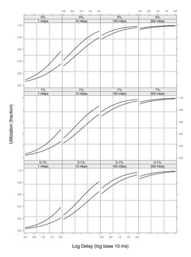
FIG. 8. The QoS utilization from the best-effort delay model graphed against log delay given the bit rate and the delay probability. The bit connection rate  $\gamma_b$  is taken to be  $2^{14}$  bits/s per connection. The upper curve on each panel estimates the expected values and the lower curve gives the minimum values of 95% tolerance intervals.
