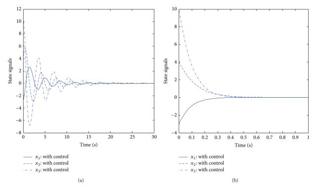
FIGURE 5: Transient response of state signals with (a) single input, single state, unit negative feedback  $u_2 = -x_2$ ; (b) static state feedback u = Kx,  $K = \text{diag} \begin{pmatrix} -10 & -10 \\ -10 & -10 \end{pmatrix}$ .
