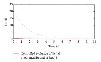
FIGURE 2: The evolution of ||x(t)|| with linear state feedback control  $u_2 = -40x_2$ . Also shown is theoretical bound of ||x(t)|| as in (7).
