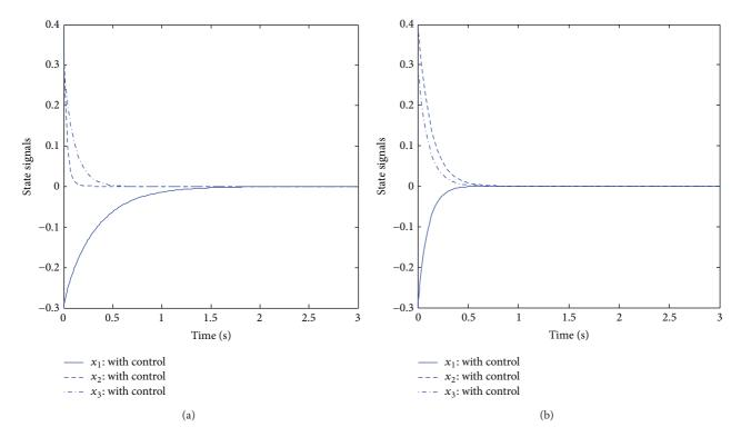
FIGURE 6: Transient response of state signals with (a) single input, single state, unit negative feedback  $u_2 = -8x_2$ ; (b) static state feedback  $u_1 = -5x_1$ ,  $u_2 = -13x_2$ , and  $u_3 = 0$ .
