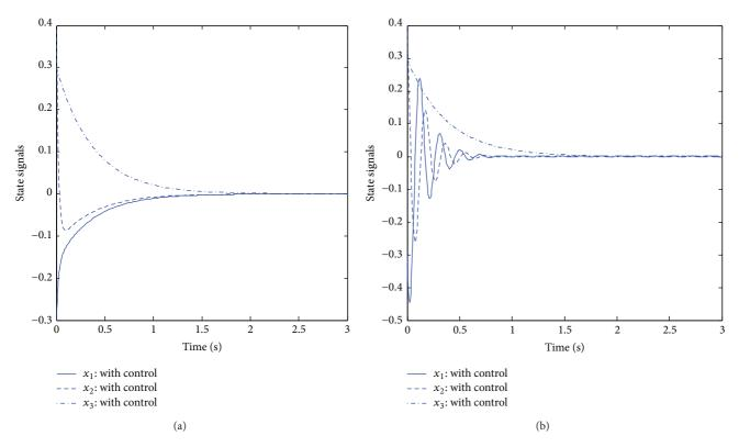
FIGURE 7: Transient response of state signals with (a) single input, single state, unit negative feedback  $u_2 = -40x_2$ ; (b) single input control  $u_1 = -2x_1 - 50x_2$ ,  $u_2 = 0$ , and  $u_3 = 0$ .
