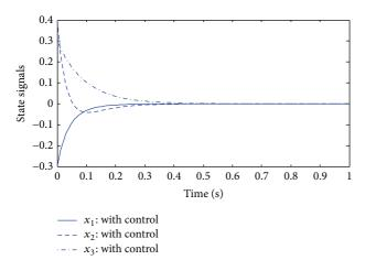
FIGURE 4: Transient response of state signals with K = diag(-20 - 20 - 10).
