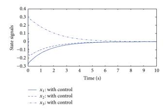
FIGURE 1: Transient response of state signals: closed loop system with  $x_0 = \begin{bmatrix} -0.3 & 0.4 & 0.3 \end{bmatrix}^T$ .
