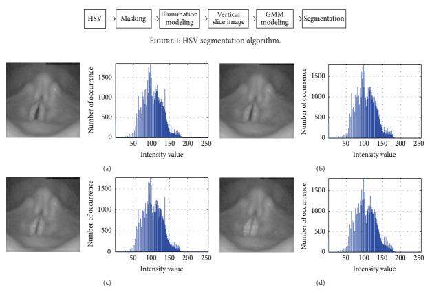
FIGURE 2: Four snapshots from HSV and corresponding histograms.
