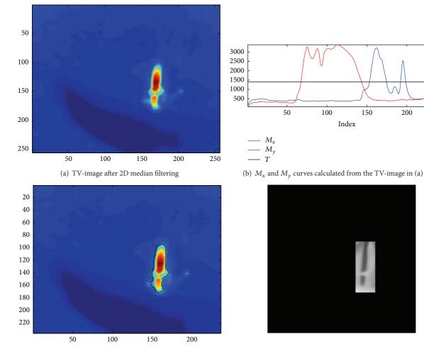
(c) The contour obtained after median filtering
