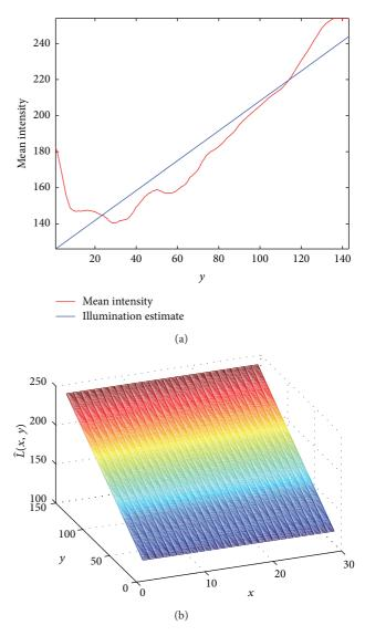
FIGURE 12: (a) Vertical slice image (VSI), intensity variation along the vertical slice of masked image. (b) Intensity variations of VSI image for different vertical lines.
