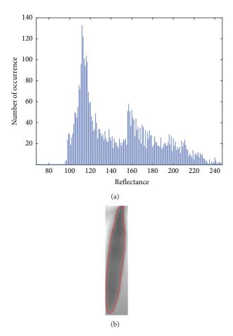
FIGURE 14: (a) Histogram of the reflectance image. (b) Estimated reflectance image and the boundary of the vocal folds obtained by thresholding with T = 150 (reflectance is scaled by 255 for grayscale representation).
