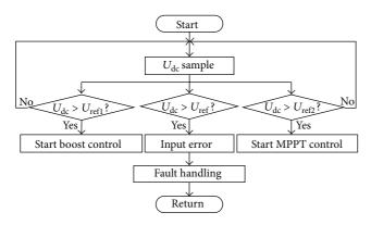
FIGURE 2: The DC/DC control flow chart.
