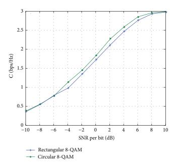
FIGURE 5: Capacity comparison between two different 8-QAM signal constellations.
