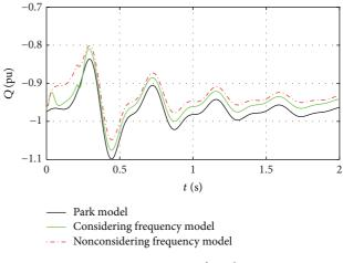
FIGURE 15: Reactive power of wind generator.
