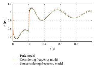
FIGURE 6: The active power of induction motor.
