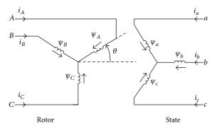
FIGURE 1: Stator and rotor circuits of an induction motor.
