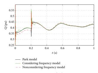
FIGURE 7: Reactive power of induction motor.
