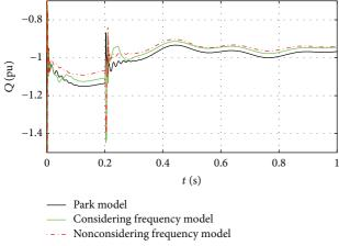
FIGURE 9: Reactive power of wind generator.
