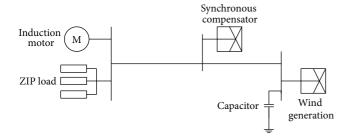
FIGURE 3: Simulation system.
