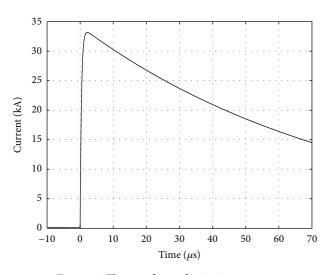
FIGURE 8: The waveform of injection current.
