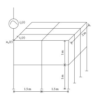
FIGURE 5: The structure diagram of a reduced-scale model.
