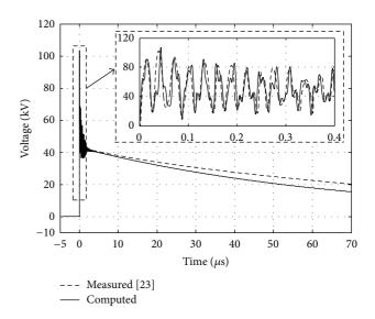
FIGURE 10: Measured and computed voltage response curves for the reduced-scale structure.
