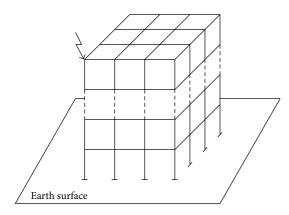
FIGURE 1: A cage-like multiconductor system.
