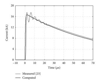
FIGURE 9: Measured and computed current response curves for the reduced-scale structure.
