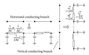
FIGURE 4: A  $\pi$ -type circuit of a two-segment subsystem.
