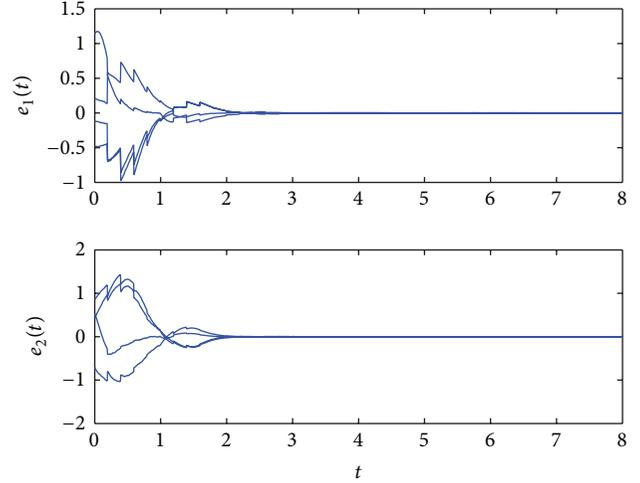
FIGURE 4: Evolution process of synchronization errors of two delayed Hopfield neural networks.
