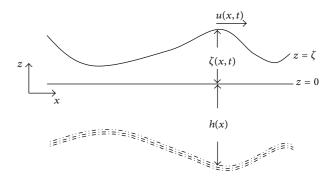
FIGURE 1: The shallow water system.
