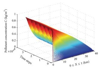
FIGURE 4: The pollutant concentration C(x, t) (mg/L) using traditional MacCormack scheme.
