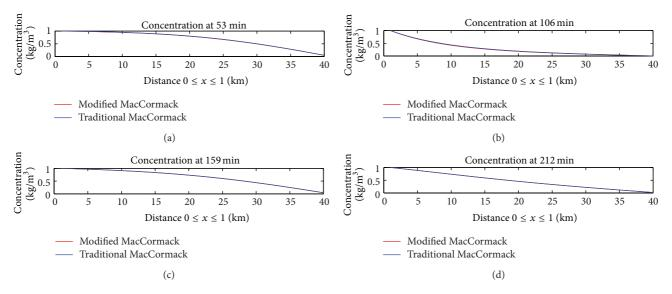
FIGURE 6: The comparison of concentration at 4 different time instants of Modified MacCormack and Traditional MacCormack methods.
