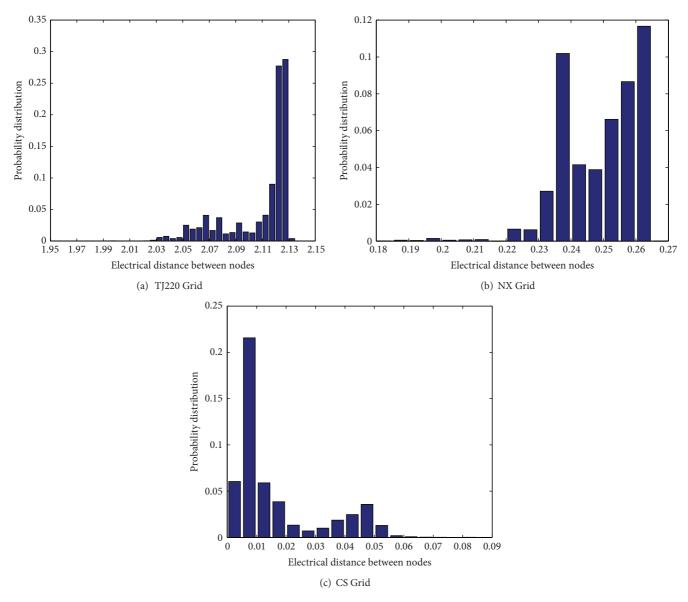
FIGURE 6: Probability distribution of electrical distance between nodes in power grids.
