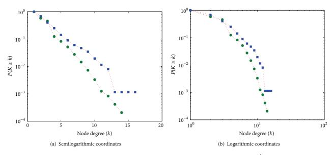
FIGURE 2: Cumulative degree distribution curves of NC Grid model  $G_{\rm NC}$  and  $G'_{\rm NC}$ .
