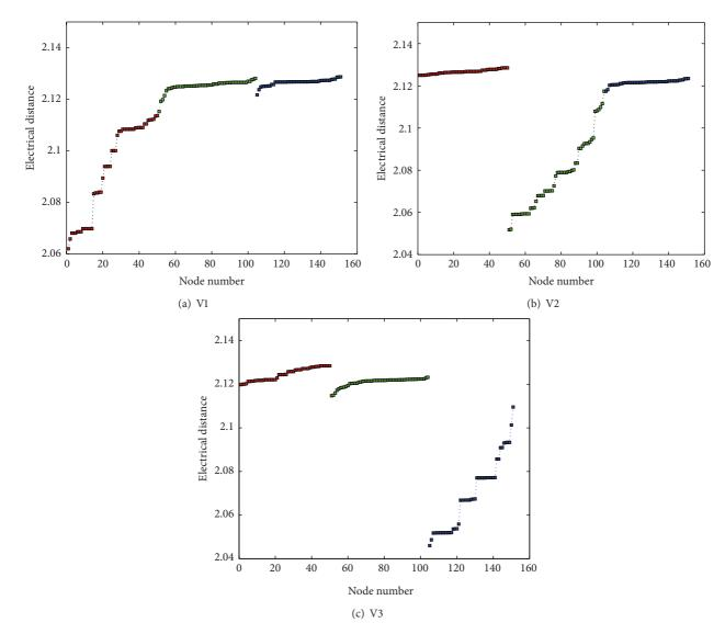
FIGURE 10: Electrical distance distribution between V1, V2, and V3 and other nodes. Red squares represent the electrical distance between the selected node and nodes in Zone1. Green squares represent the electrical distance between the selected nodes and nodes in Zone2. Blue squares represent the electrical distance between the selected node and nodes in Zone3.
