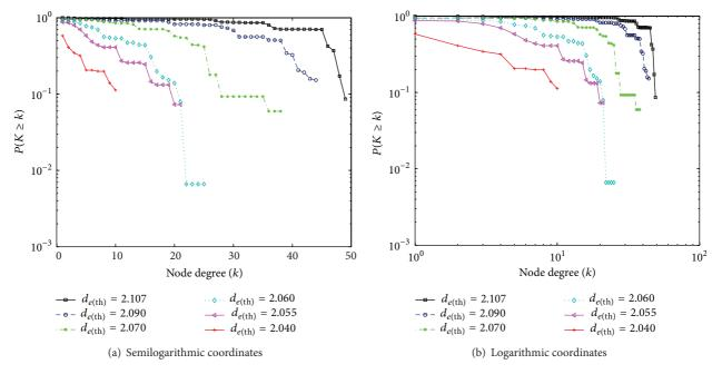
FIGURE 8: Cumulative degree distribution of electrical distance-based network model of TJ220 Grid.
