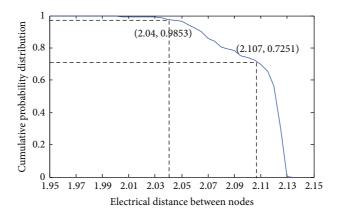
FIGURE 7: Cumulative Probability distribution of electrical distance between nodes in TJ220 Grid.
