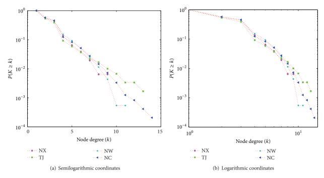
FIGURE 1: Cumulative degree distribution of topology-based model of power grids.
