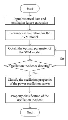
FIGURE 4: Flow chart of the oscillation property classification.
