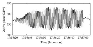
FIGURE 6: The active power oscilloscope record of Yao-Shao tie line.
