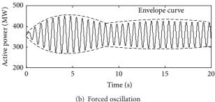
FIGURE 1: Power oscillation curve of tie line.
