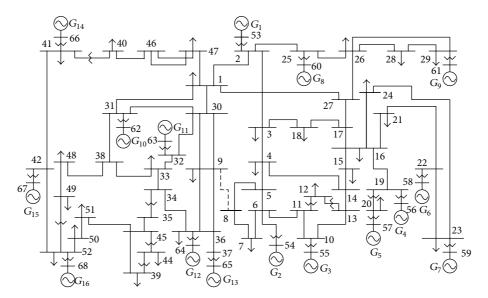
FIGURE 5: Simulation example of IEEE16-machine 68-bus benchmark system.
