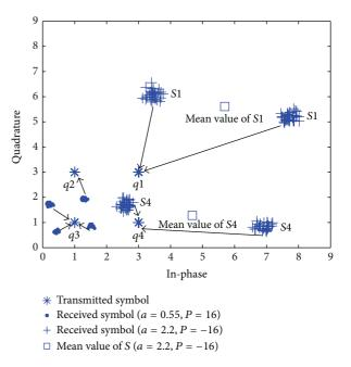
FIGURE 2: Square 16QAM symbols with different fading coefficients (first quadrant).
