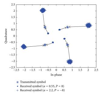
FIGURE 1: QPSK symbols with different fading coefficients.
