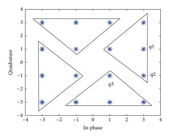
FIGURE 4: Subsets of square 16QAM constellations.
