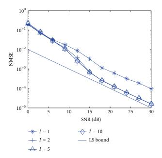
FIGURE 9: NMSE comparisons of ML-LM iteration for different numbers of iterations.
