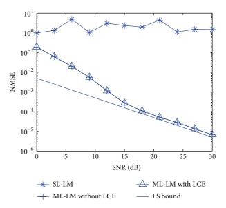
FIGURE 8: NMSE comparisons of SL-LM and ML-LM iteration when L = 200 (with and without LCE).
