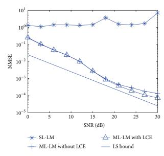
FIGURE 6: NMSE comparisons of SL-LM and ML-LM iteration when L = 40 (with and without LCE).
