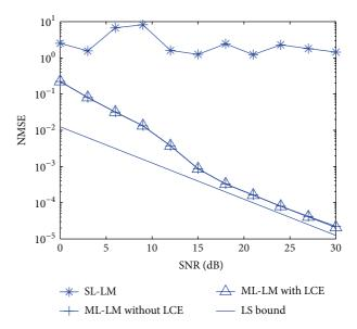
FIGURE 7: NMSE comparisons of SL-LM and ML-LM iteration when L = 80 (with and without LCE).
