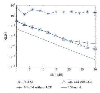
FIGURE 5: NMSE comparisons of SL-LM and ML-LM iteration when L = 20 (with and without LCE).
