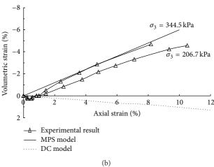
FIGURE 1: Calculation and test results for triaxial test of Ottawa silica sand.
